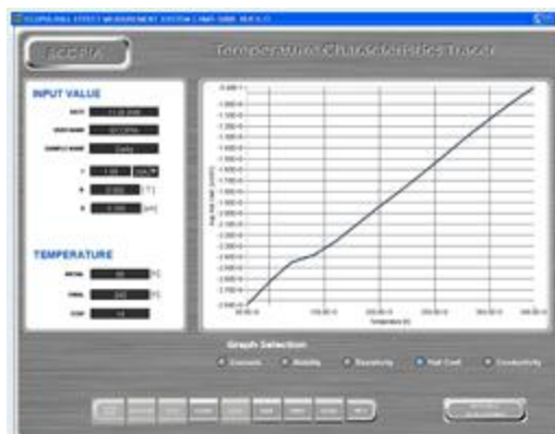
Hall Coefficient vs temp variation
