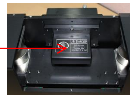
< Automatic magnet movement (0.55Tesla magnet) >
