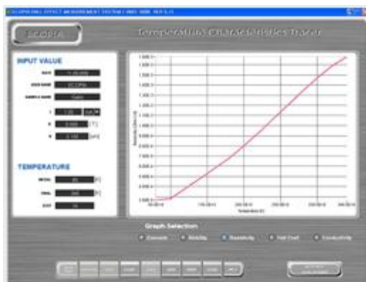
Resistivity vs temp variation
