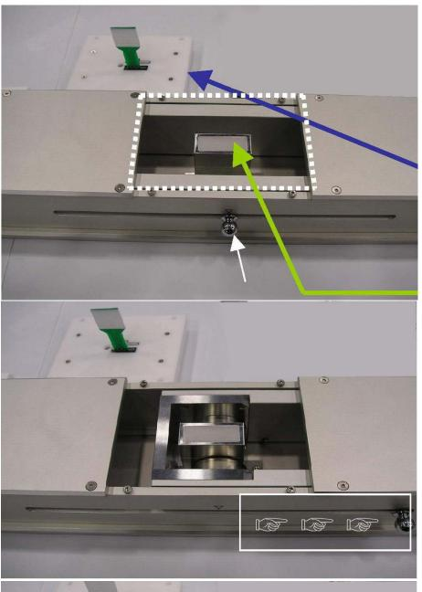
This image shows the sample mounted on a board and installed in the sample lid, but not yet installed into the MP55T sample kit. The blue arrow is pointing to the board mounted sample in the lid.
