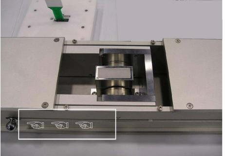
Here the knob (see hands pointing) has been moved to the far left position, placing the magnet field in the south → north orientation.
