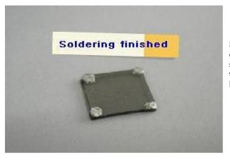
Sample, ready to be mounted onto the spring clip mounting system, or to be wired using the sample board for wire bonding samples.
