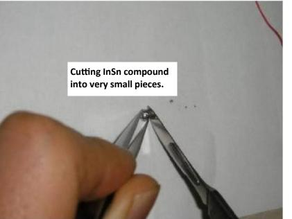
Using a razor blade knife, cut tiny fragments of the cooled InSn so that it can be applied to the corners of the sample.
