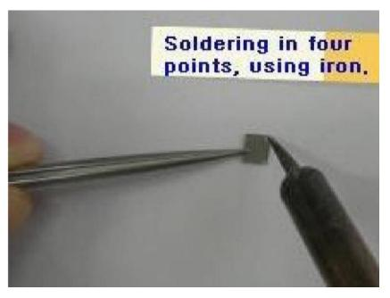
Use the soldering iron to melt the InSn into the four corners of the material. It should be done as close to the corner as possible. If the sample has not been annealed, it might be helpful to keep the soldering iron in contact for about one minute to improve ohmic contact.
